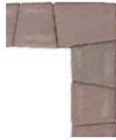
'Solid Wall' construction
